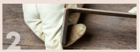
The finished bend should have a nice sharp corner, without any cracks along the outside. If you attempt to bend too thick a section, it will require considerable force, and cracks will form along the outside of the corner.
