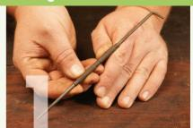
A scriber is the first place to start because it is used to make accurate marks or scratches on metal. While there is nothing wrong with using a pencil or marker pen for basic marking out, if you want accuracy better than plus or minus a millimetre a scriber is the tool to use. This scriber has a straight end for general marking and a bent end for access in restricted spaces. Scribers are sharpened to a fine, sharp point on a bench grinder.
