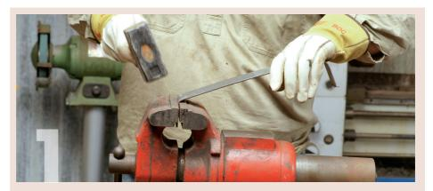
Flat bar can often be bent in the bench vice by clamping firmly, and then striking the bend with a hammer as the steel is pulled over with the other hand.
